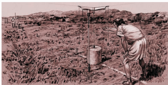
Figure 3. Recreation of land plots around Ilici being surveyed using a groma . The Crevillente Mountains are in the background.
