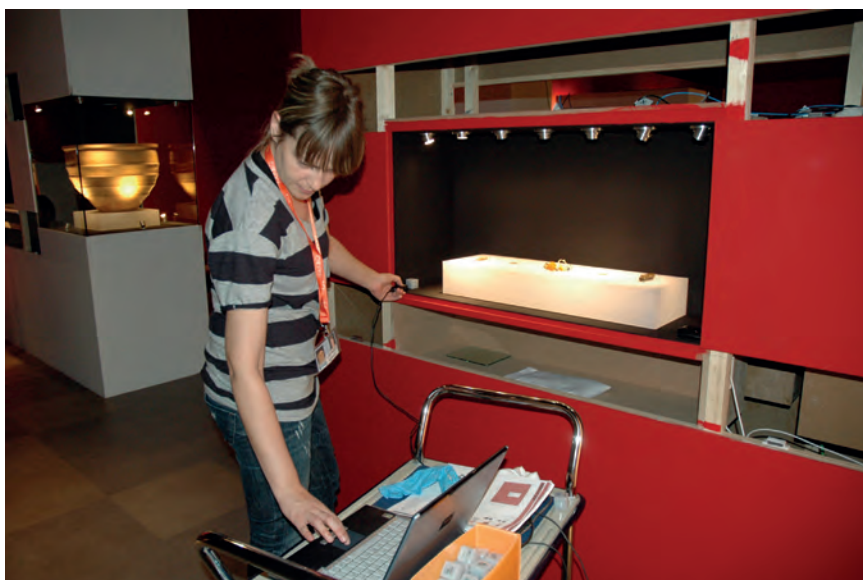
Fig.6. Use of data logger infrared lights to check humidity and temperature levels. Used for climate control during temporary exhibitions. MARQ graphics archive.
